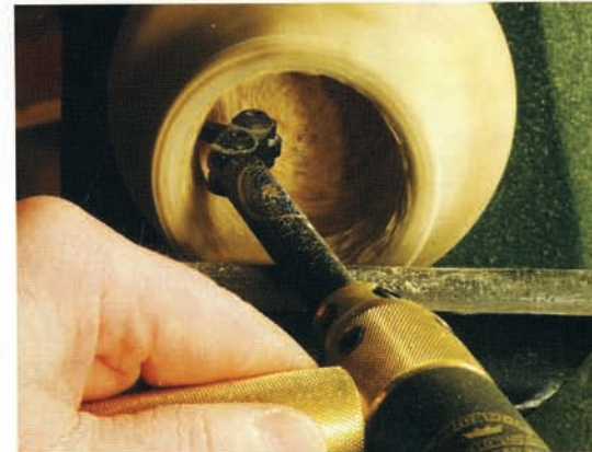
ABOVE: Side handle being used when rough shaping. This brass section can also be used in the end of the handle as an extension piece
