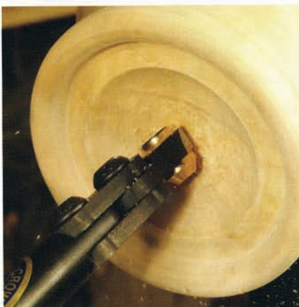
ABOVE: Super Ring Cutter in use with the cutter tilted to achieve a shearing cut
