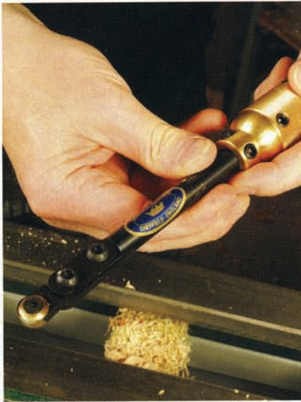
ABOVE: Hollowing tool shaft into handle collet
